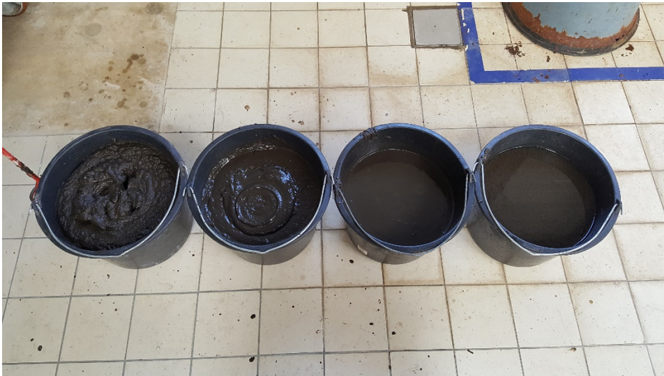
Figure 2. Photograph of Typical Thickened Solids at Varying Concentrations (from left to right: 8.25% solids, 6.0% solids, 3.2% solids, and 1.0% solids)
