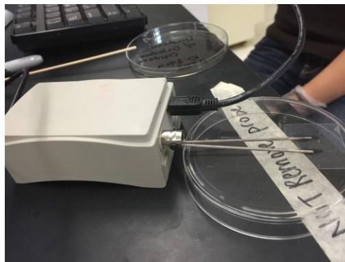
Photo by Author Fig. 3 Biosensor connected to eDAQ ammeter via Pt/Ti counterelectrodes
