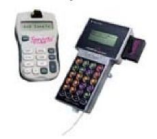
Figure 10. Spreeta Chip Mounted in a Field-Portable Readout Module. (Sensata 2008)
