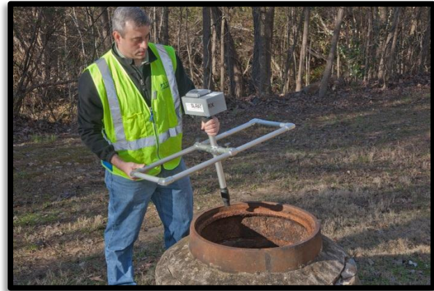
The Sewer Line Rapid Assessment Tool, aka the SL-RAT, from InfoSense, Inc.
