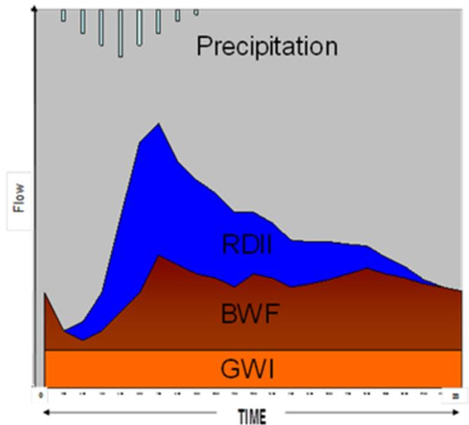
Figure 2: Components of wet-weather wastewater flow during a precipitation event. (US EPA, 2007)
