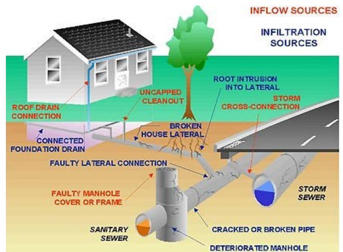
**Figure 1:** Typical sources of I/I in sanitary sewer systems.
