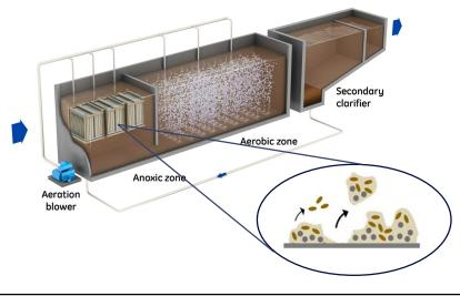
hybrid system with nitrification in biofilm and suspended biomass
