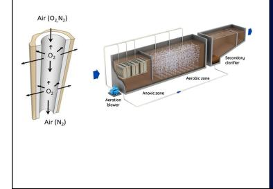
O<sub>2</sub> is delivered by molecular diffusion – without bubbles
