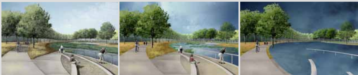
FIGURE 5-60 Illustrations show consolidated treatment areas in proposed parks. The image on the left illustrates the fair weather condition, the center image the water quality capture volume, and the image on the right the 100-year storm event. Construction was completed in spring 2007.
