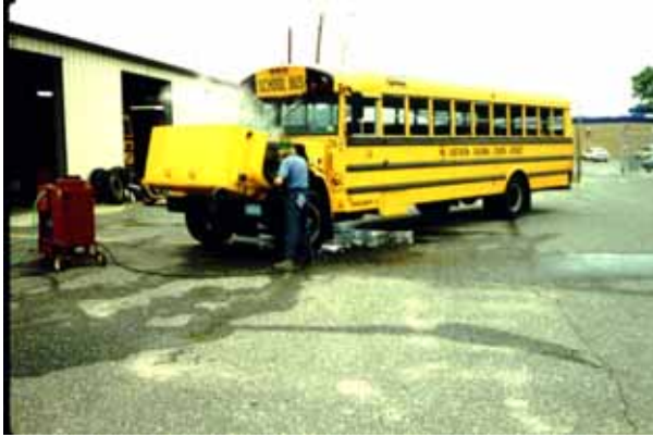
Washing of vehicle engine and allowing runoff to enter storm drainage system. SOURCE: Robert Pitt.
