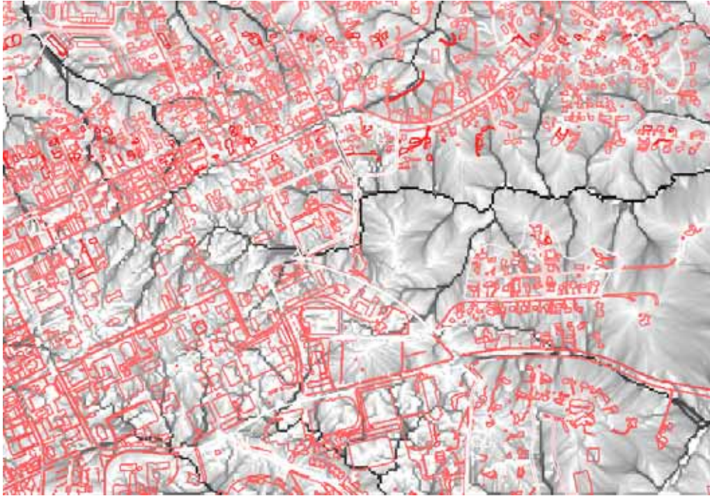
FIGURE 4-15 A small urban catchment in the Lake Jordan watershed of North Carolina with distributed sources of impervious surface (buildings and roads) stormwater arranged within the full surface drainage flowpath system. Stormwater from each source is routed down surface and subsurface flowpaths to the nearest tributary and out the drainage network, with additions and abstractions of water and pollutants along each flowpath segment.
