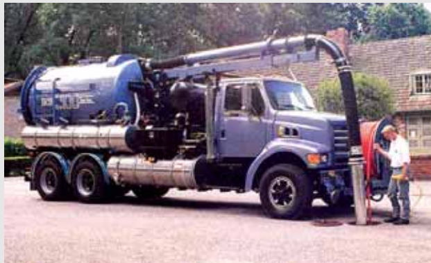
FIGURE 2-3 Catch basin cleaning. Courtesy of Robert Pitt.
