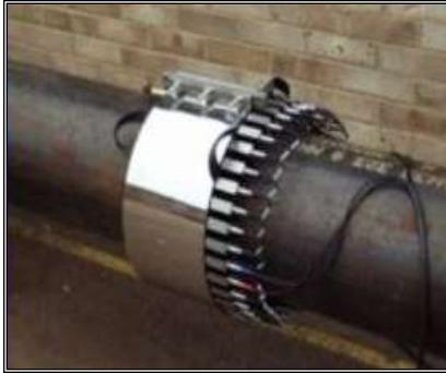
**Figure 5-11. Example wrap-around collar with piezoelectric shear motion sensor (Teletest sensor collar).**
