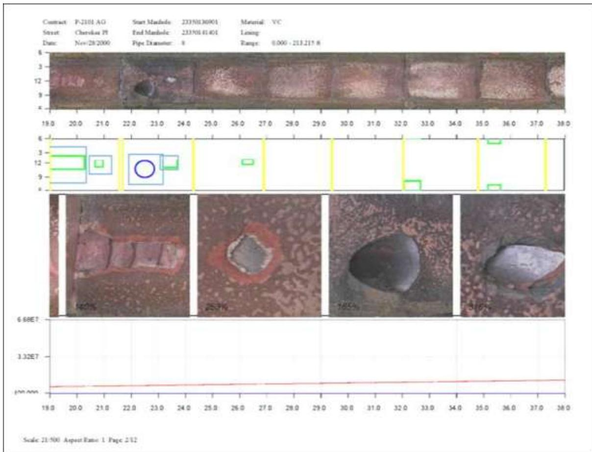
**Figure 4-4. Example of side scanning results**
