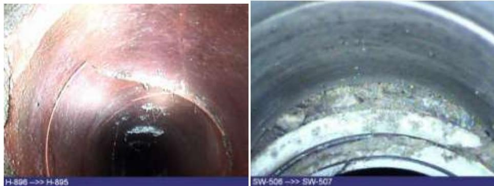
**Figure 3-4. Zoom camera images of pipes showing structural defects.**
