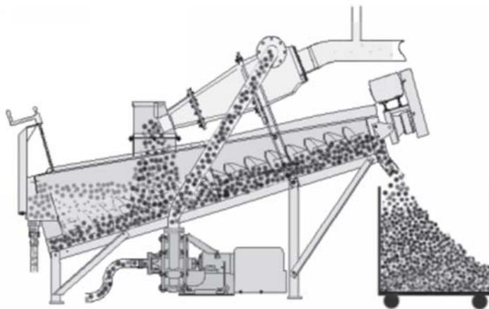
Figure 5: Cyclone and Classifier (Wemco, Inc.)
