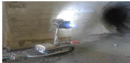
Figure 10 – An example of a crawling ROV which is inspecting the structural integrity of the tunnel. (Photo: Courtesy of Redzone Robotics, ASI Marine)
