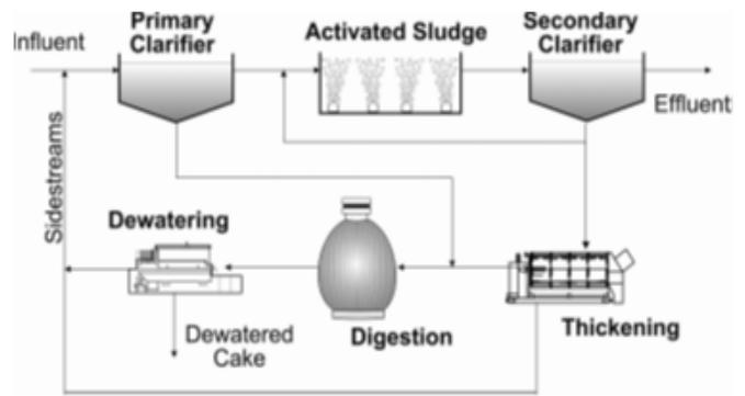
Figure 2 - Example model flow schematic showing process flow linkages between unit processes.
