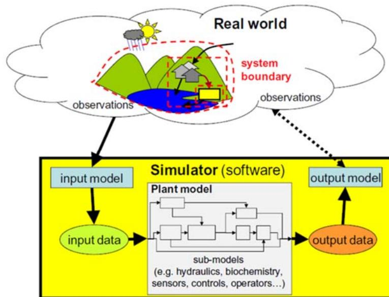
*Figure 1 – Connection between real world observation and a plant model (Guidelines for Using Activated Sludge Models, Figure 2.2)*
