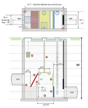
Figure 12 – Design for NEORSD's Near Surface Facilities which are installed at each drop gate along new tunnels. (Figure provided by NEORSD)
