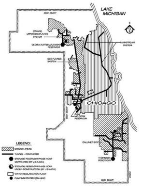
Figure 4 – Map of the MWRDGC's TARP service area. (Figure provided by: MWRDGC)
