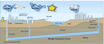
Figure 2 – An overview of deep tunnel systems for CSO control. (Figure provided by F. Oksuz)
