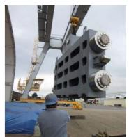
Figure 14 – High head wheel gates for tunnels. (Photo provided by F. Oksuz)
