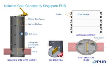
Figure 9 – Roller isolation gates concept developed by Singapore PUB. (Figure provided by Singapore PUB)
