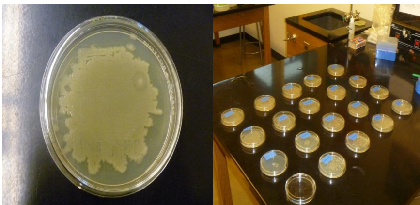
Figure 4: Bacterial culture in a petri dish (left) and array of all petri dish samples (right) used to determine the toxicity of the control and sulfidized samples
