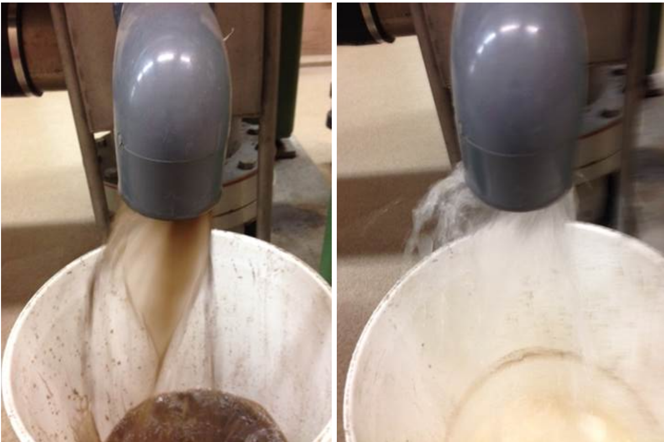
Figure 5. Visibly Poor Filtrate (on Left) Compared to Visibly Clean Filtrate (on Right)
