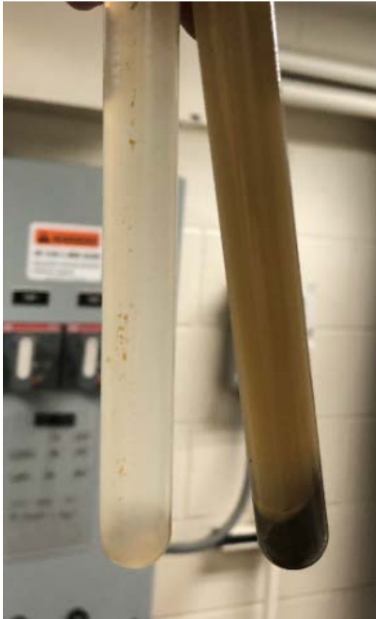
Figure 4. A Laboratory Centrifuge Can Provide a Quick Indication of Solids Capture Reprinted with permission from GEA Mechanical Equipment US, Inc., GEA Westfalia Separator Division
