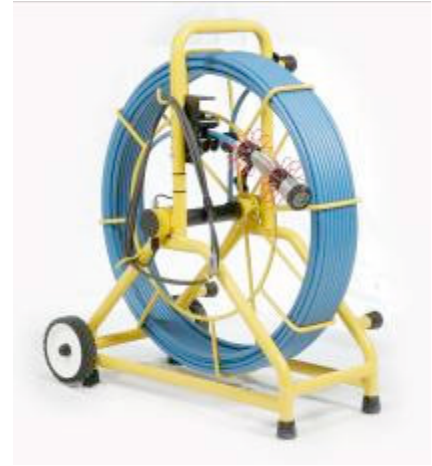
Figure 2-15. Crystal Cam – push camera. Image courtesy of Inuktun Services, Ltd.
