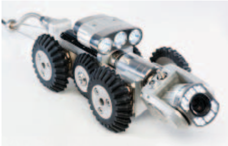
Figure 2-13. Mobile robot inspection system. Source: iPEK International GmbH (2009). Reprinted with permission.
