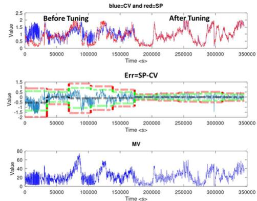
Poor tuning and bad data prevent ability to track set points. Well-tuned controllers perform better.
