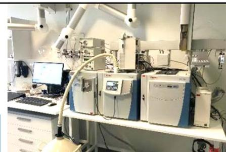
Methane was measured by GC-FID. VFA and sulfate was measured using ion chromatography
