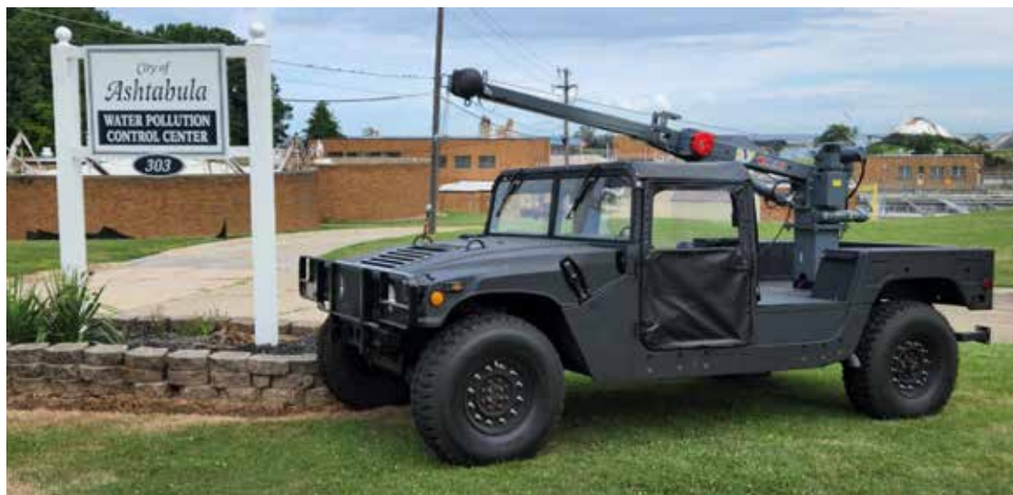
Staff members at the City of Ashtabula (Ohio) Water Pollution Control Center retrofit a Humvee with an electric-hydraulic service crane to help with collection system and facility maintenance.
