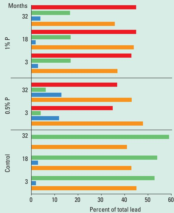
We conclude that in situ addition of phosphate to lead-contaminated soil under field conditions can alter the form of soil lead and its bioavailability and that it is possible to measure the bioavailability of soil lead using animal bioassays and simple chemical in vitro techniques. Thus, we proved that under field conditions, in situ soil treatments change the form of soil lead and its bioavailability. The apparent environ-
