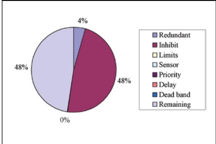
**Figure 4. Alarm Occurrences Within a 7-Day Period (by Frequency)**
