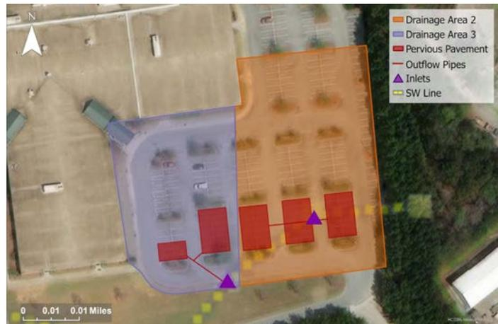
Figure 11: Alternative 2 Drainage Areas for Pervious Pavement (Esri, n.d.; Gwinnett County GIS, 2020)
